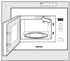
Stick the included short instructions to the frame behind the door (as shown). Be sure not to block the vents. Microwaves:
